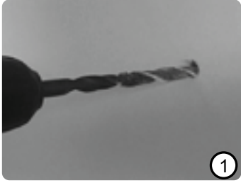
1. Drill the hole for screws (4mm screw diameter)
