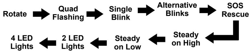
To turn off the warning light without cycling through the 9 light modes, press and hold the power button for 2 seconds. Two LEDs will flash five times and then turn off. When ready to operate again, press the power button once and it will return to the last flash mode that was selected before turning off.
