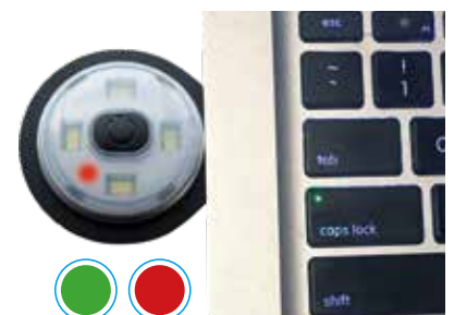
The charging indicator will glow red while charging and turn green once charged
