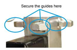
② Its recommended to use the supplied guide lines to secure the tripod on ruff terrain or harsh weather conditions.
