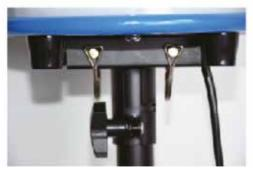
**3** Open the tripod bracket and align the hole with tripod fitting, then attach the safety bolt and tighten it.
